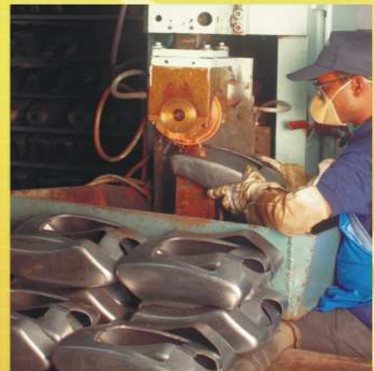
MESH & SEAM WELDING MACHINES "MECHLONIC" make mesh and seam welding machines to manufacture 100% leak free Petrol tank for any type of two - wheeler vehicles.
